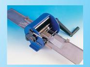
The model SEF 1 is designed for separating wires of flat cables. Two different pitches of separation can be supplied: 1,27 mm (the wires are individually separated Code 73.0L01) 2,54 mm (the wires are separated by couples Code 73.0L02). This version is a "bench" manual machine suitable for separating edges of flat cables having maximum width of 66 mm. Motor drive unit cod. 61.0L01 (110 volt) cod .61.OL02 (220 volt)
